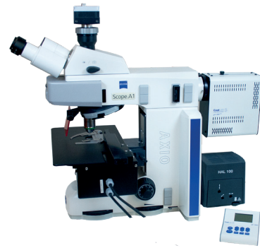
Microscope with fluorescence equipment
